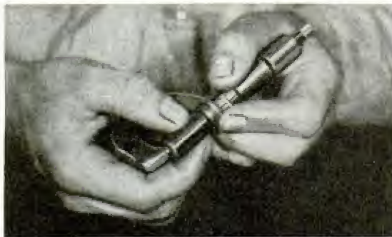
SQUARING WORN CONTACT OF ANVIL WITH IMPROVED ALIGNING SLEEVE
